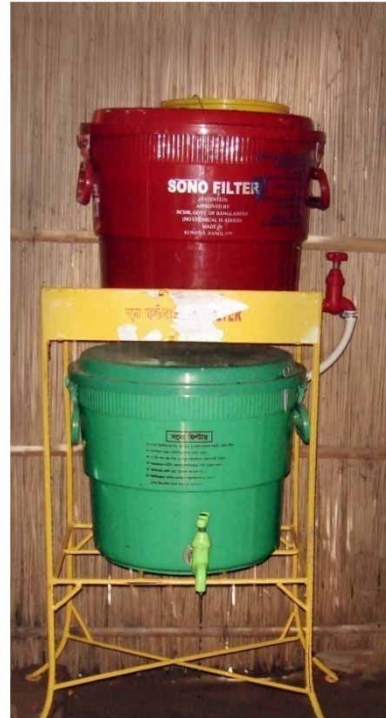
Fig. 2. Schematic diagram of Sono 2-bucket filter (Hussam et al. , 2008) (left); picture of Sono filter taken by one of the authors (right).
